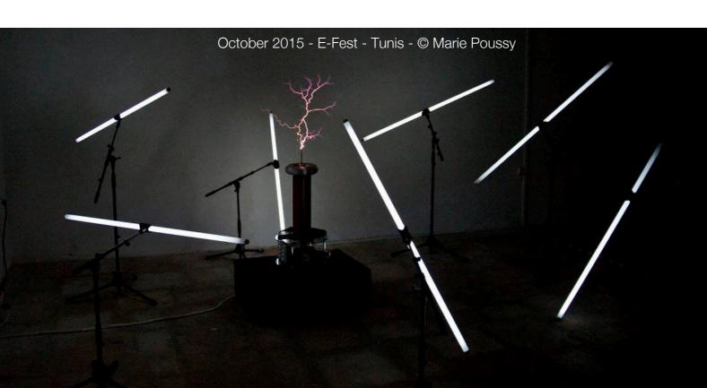
The Tesla coil is run with a MIDI controller by a computer which generates sequences which replicate recordings of electromagnetic pulses in the immediate vicinity. It reacts to the presence of the audience. The sound is run via the spark outputs. A MIDI sequence of 30 seconds is triggered by the approach of a spectator, every 5 minutes. 8 to 10 fluorescent tubes hung on stands are placed around the space, and the fluorescents are powered by the electromagnetic fields coming from the coil.
